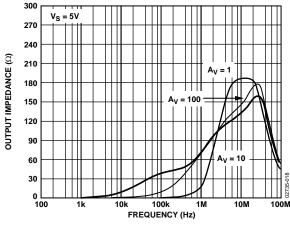
Figure 22. Output Impedance vs. Frequency at 5 V
