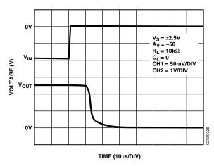
Figure 30. Negative Overvoltage Recovery
