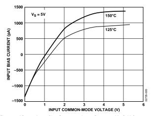
Figure 9. AD8628 Input Bias Current vs. Input Common-Mode Voltage at 5  $\rm V$
