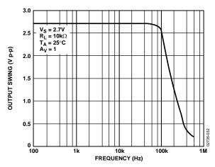
Figure 36. Maximum Output Swing vs. Frequency
