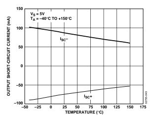
Figure 47. Output Short-Circuit Current vs. Temperature
