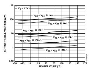
Figure 49. Output-to-Rail Voltage vs. Temperature
