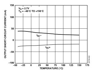
Figure 46. Output Short-Circuit Current vs. Temperature
