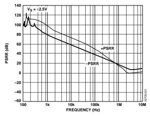
Figure 35. PSRR vs. Frequency
