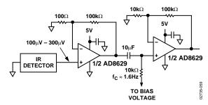
Figure 64. AD8629 Used as Preamplifier for Thermopile
