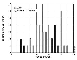
Figure 11. Input Offset Voltage Drift
