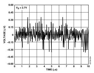
Figure 38. 0.1 Hz to 10 Hz Noise at 2.7 V
