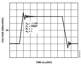
Figure 23. Large Signal Transient Response at 2.7 V
