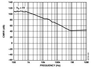
Figure 33. CMRR vs. Frequency at 5 V
