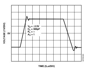
Figure 24. Large Signal Transient Response at 5 V
