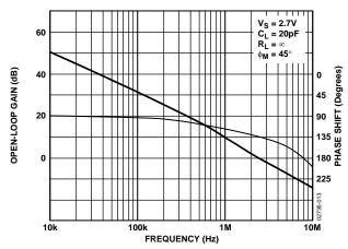
Figure 17. Open-Loop Gain and Phase vs. Frequency
