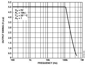
Figure 37. Maximum Output Swing vs. Frequency at 5 V
