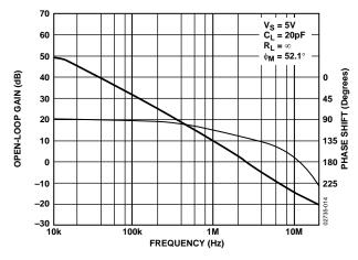
Figure 18. Open-Loop Gain and Phase vs. Frequency
