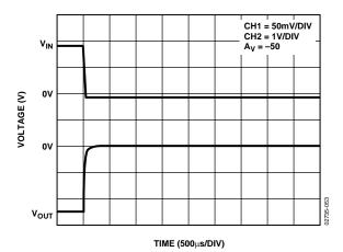
Figure 58. Positive Input Overload Recovery for the AD8628
