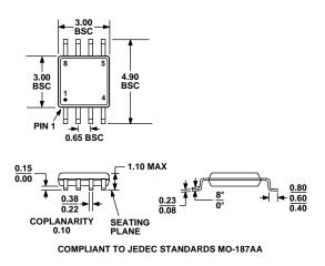
Figure 70. 8-Lead Mini Small Outline Package [MSOP] (RM-8) Dimensions shown in millimeters
