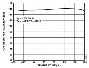
Figure 45. Power Supply Rejection vs. Temperature
