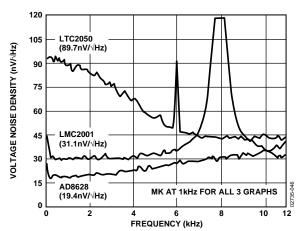
Figure 51. Noise Spectral Density of AD8628 vs. Competition
