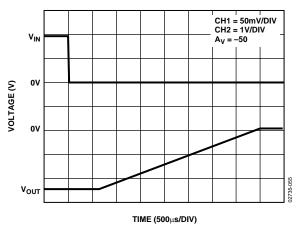
Figure 60. Positive Input Overload Recovery for LMC2001
