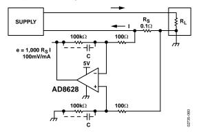
Figure 65. Low-Side Current Sensing
