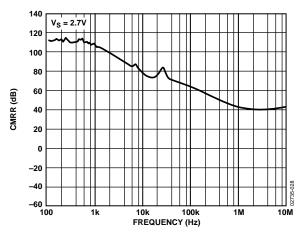
Figure 32. CMRR vs. Frequency at 2.7 V
