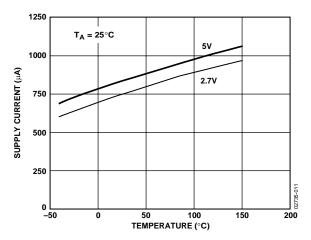
Figure 15. Supply Current vs. Temperature
