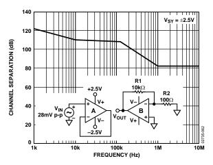
Figure 50. AD8629/AD8630 Channel Separation
