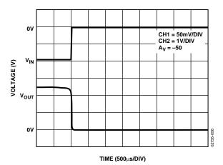
Figure 61. Negative Input Overload Recovery for the AD8628
