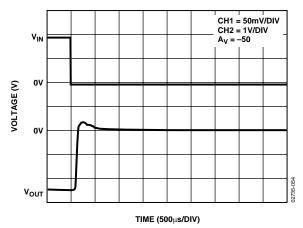
Figure 59. Positive Input Overload Recovery for LTC2050
