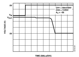
Figure 62. Negative Input Overload Recovery for LTC2050
