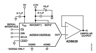
Figure 66. AD8628 Used as an Output Amplifier
