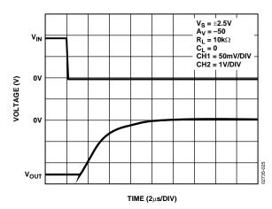
Figure 29. Positive Overvoltage Recovery
