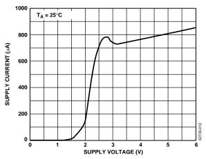
Figure 16. Supply Current vs. Supply Voltage
