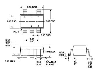
\*COMPLIANT TO JEDEC STANDARDS MO-193-AB WITH THE EXCEPTION OF PACKAGE HEIGHT AND THICKNESS.
