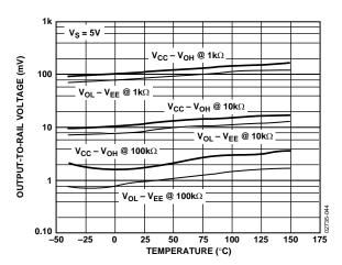
Figure 48. Output-to-Rail Voltage vs. Temperature
