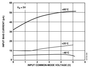
Figure 8. AD8628 Input Bias Current vs. Input Common-Mode Voltage at 5  $\,\mathrm{V}$
