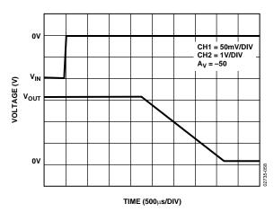
Figure 63. Negative Input Overload Recovery for LMC2001
