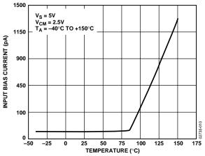
Figure 14. AD8628 Input Bias Current vs. Temperature
