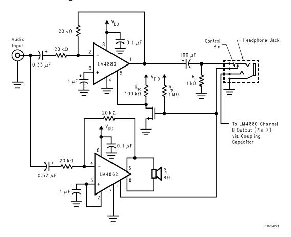
FIGURE 2. Automatic Switching Circuit
