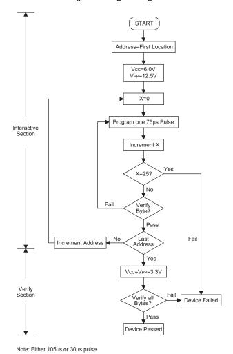
Figure 3. Fast Programming Flowchart
