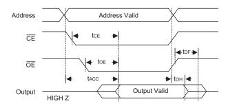
Figure 1. A.C. Waveforms for Read Operation
